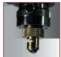
5mm Steel Swivel nose cone for 11/64" cutters. For glass engraving and to control depth on uneven or curved surfaces Part no. 20459
