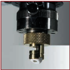
3.5mm Teflon Swivel nose cone for 11/64" cutters. For glass engraving and to control depth on uneven or curved surfaces - prevents scratches. Part no. 22481
