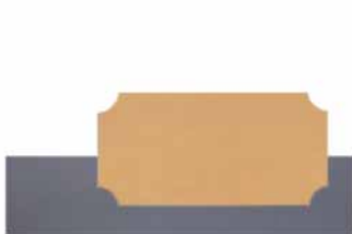
Cutting of concave corners
