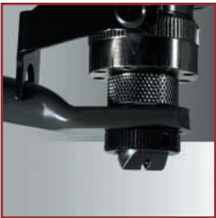
Prismatic Swiveling Steel nose cone for 11/64" cutters. Used for curved jewelry-bracelets such as ID or bangle bracelets Part no. 22885
