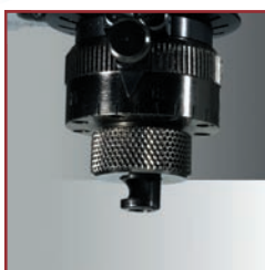
.250 Steel nose cone for 1/4" cutters. Uses up to .187 cutter widths Part no. 20491
